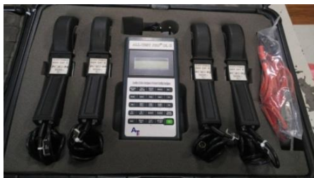
Gambar 2.5 ESA ( Electrical Signature Analyzer ) ALL-TEST PROC OL II
