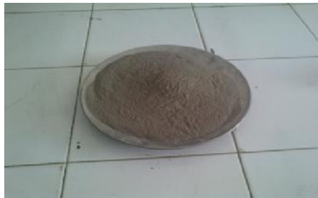
Gambar 2. Hasil Abu Cangkang Sawit lolos # 200
