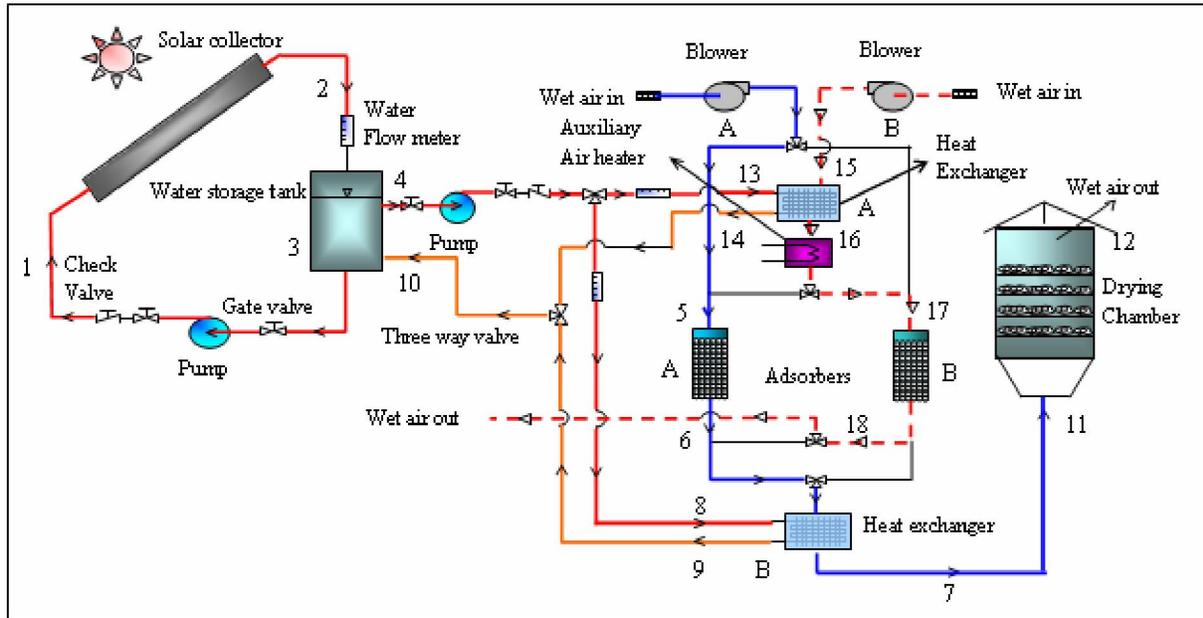
Figure1. Schematic diagram of the solar assisted dehumidification drying system
