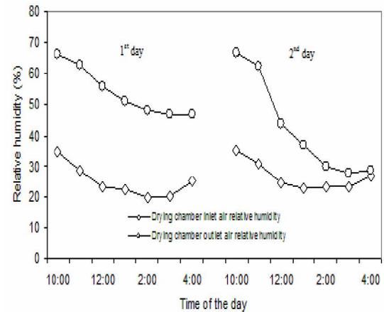
Fig.4. Variations of drying chamber inlet and outlet air relative humidity with time.
