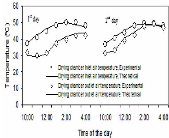
Fig.3. Variations of drying chamber inlet and outlet air temperatures with time.
