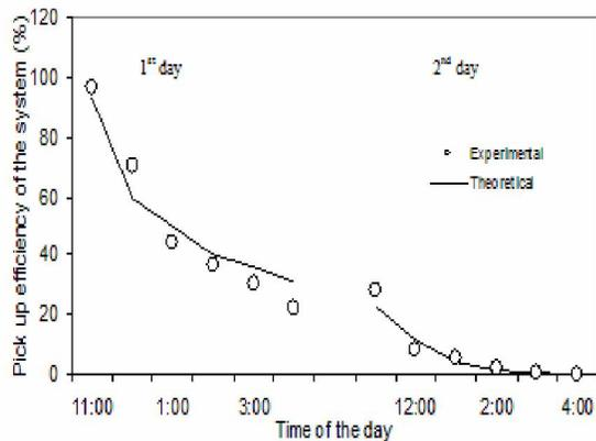
Fig.6. Variations of pick up efficiency of the system with time
