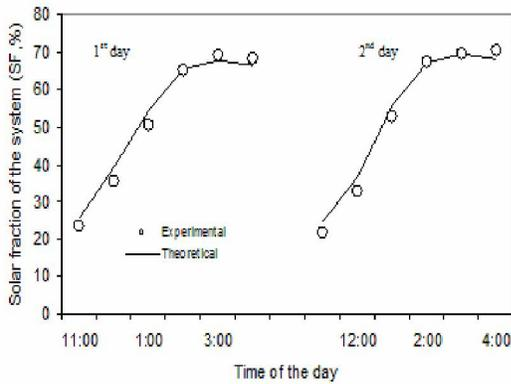
Fig.11. Variations of solar fraction of the drying system (SF) with time.
