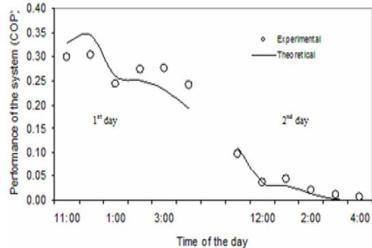
Fig.10. Variations of coefficient of performance of the drying system (COP) with time.
